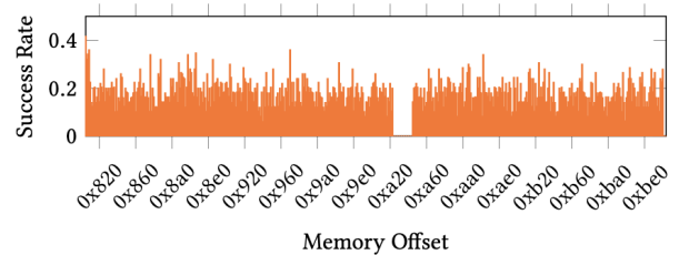
Fig. 2. Using the low success probability of rowhammer to correctly guess the start of the .text section (despite the presence of KASLR) in HammerScope [3].
